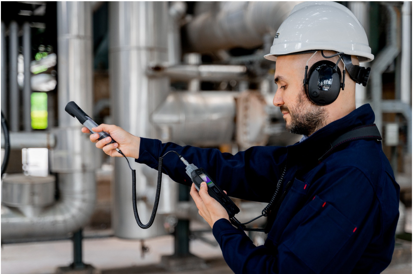
A Repower employee listens to a customer's compressed air system for possible leaks.
